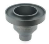
The process of flow through an orifice can often be used as a relative measurement and classification of viscosity. This measured kinematic viscosity is generally expressed in seconds of flow time which can be converted into Centistokes using a viscosity disc calculator. Viscosity Flow Cups are used for measuring the consistency of paints, varnishes and other similar products.
